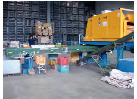
Matec has adopted and adapted new technologies for processing e-scrap. It has acquired, among other machines, a Steinert eddy-current separator for sorting shredded e-waste and utilises flotation technology for the separation of plastics.
