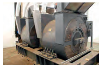
Supplied by Quad Plus, two 2000 HP DC motors at Hawkeswood Metal Recycling.
