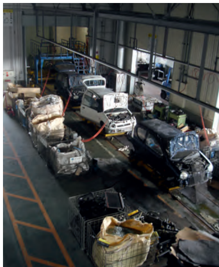
Crashed cars are being dismantled in one of the company's several ELV warehouses.
