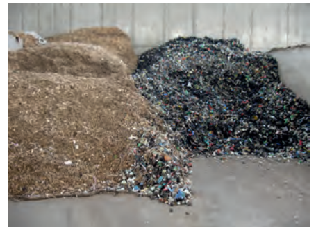
Matec runs its own automotive shredder residue separation plant. What can't be separated is eventually combined with shredded plastics and wood chips, and manufactured into high-quality fuel pellets sold to paper mills.
