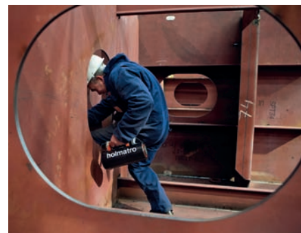
Holmatro's new double-acting aluminium cylinder allows workers to lift 100 tonnes on their own.
