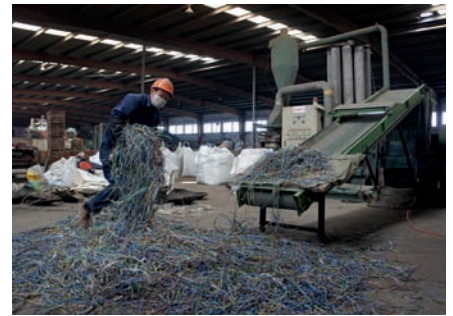
In the wire stripping area, a worker gathers a pile of fine wires by the armful and places it onto a conveyor that feeds into one of the company’s granulators.
