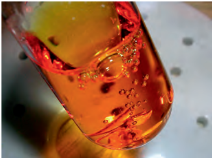
Pure platinum wire (99.95 %) dissolves easily in a mixture of one part nitric acid, two parts hydrochloric acid.
