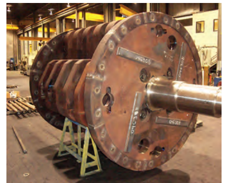
A spider rotor of a 98-inch diameter mill in the assembly hall. The spiders and discs are capped with cast steel.
