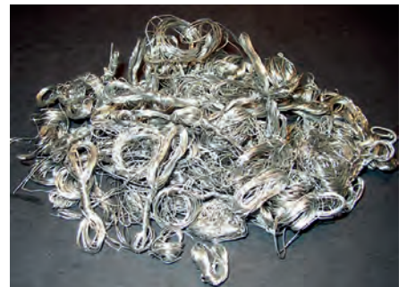
Type R and Type S platinum - rhodium thermocouple wire.
