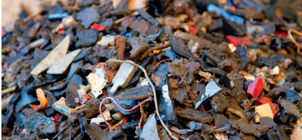
Plastics mixture in automotive shredder residue.
