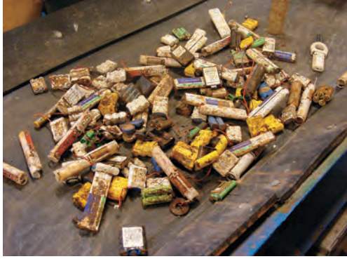
Corroded batteries are very hard to recycle.
