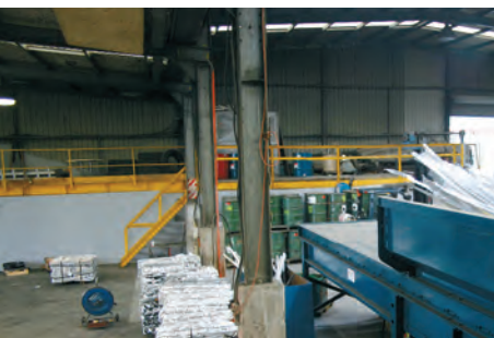
The AGP-220 can be fitted with a feed table of up to 8 metres/315 inches in length.
