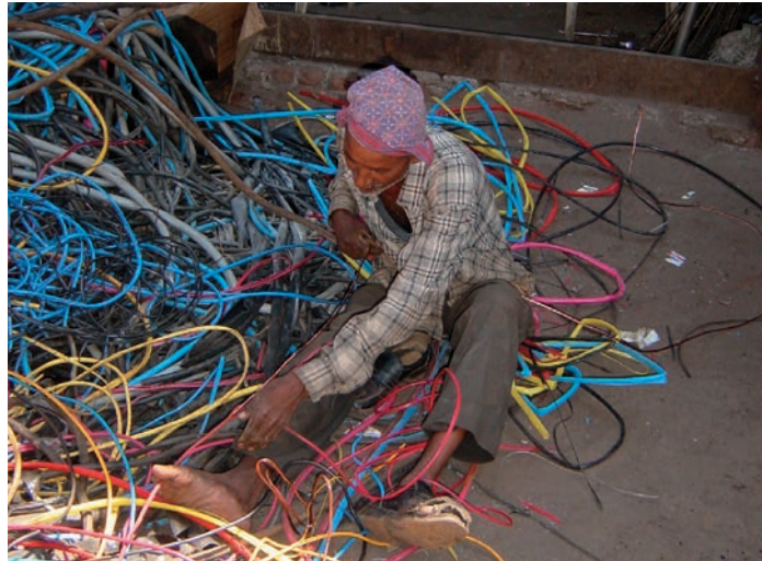
Cables are stripped by hand.
