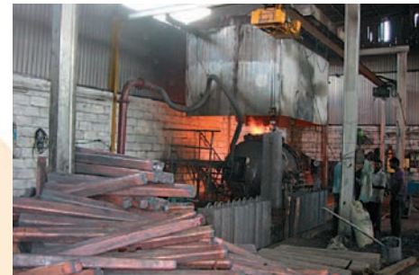
This Scalnar copper furnace has a capacity of six tonnes per hour.
